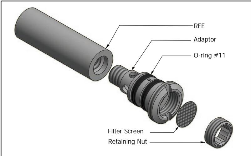
5. Clean or replace each of the removed parts as necessary. If alcohol is used for cleaning, allow time for drying.
